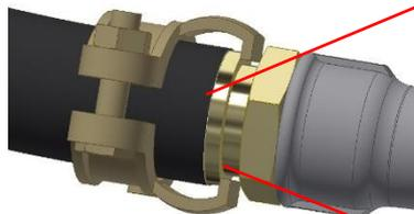
Hose must be pushed up to the collar of the hose nipple.
